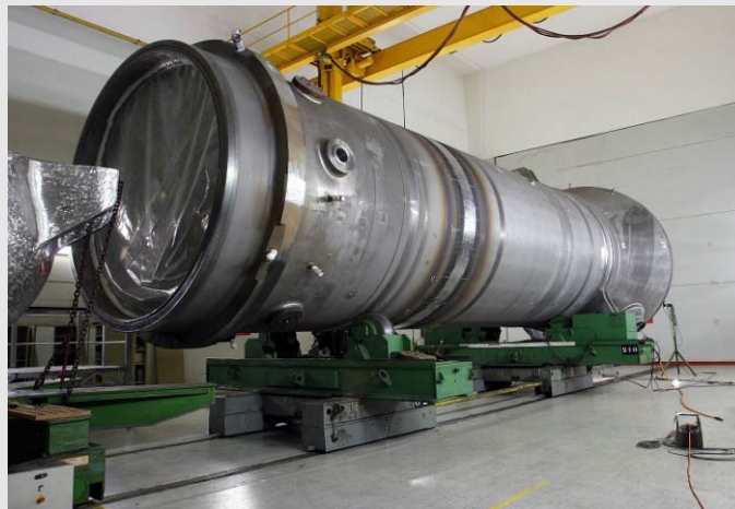
Steam Generator Lower Pressure Boundary Subassembly
