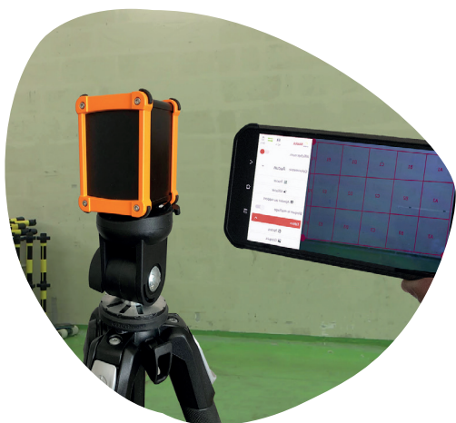
Deployment of MARA in the field: definition of a regular mesh on a wall
