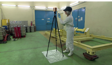
Installation of the MARA box on a tripod
