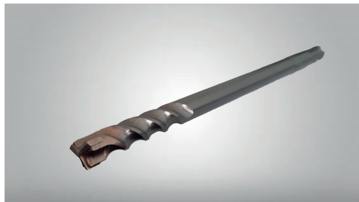
Drill adapted to capture particles by the gel
