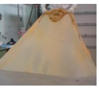
Strippable resins can be used to protect, contain or decontaminate equipment and premises. These resins consist of a sprayable gel forming a strippable film after crosslinking.
