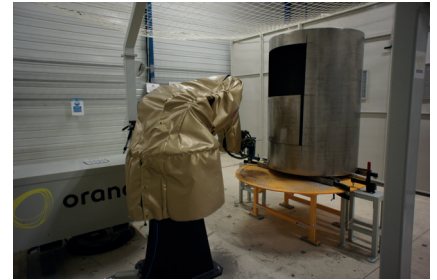
Representative model of an ECE drum from Orano la Hague
