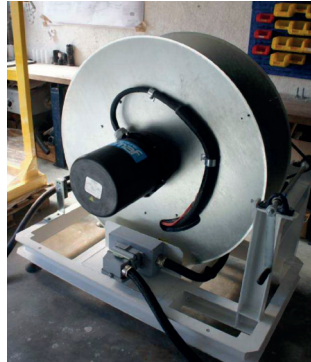
Power and control cable of the RODSY10+ rover
