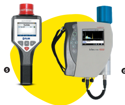
Examples of mobile spectrometers, used during dismantling projects or by first responders (fire brigade)
