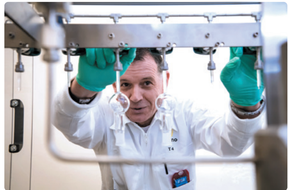
Filling a 85Kr ampoule
