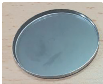
1.9 in (47 mm) diameter planchet provided by the customer
