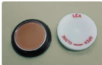
1.6 in (40 mm) active diameter source deposited in 1.9 in (47 mm) diameter customer planchet.
