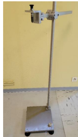
Support essais de chocs et poinçonnements Shock and punching test support
