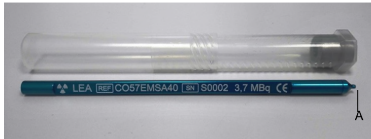
Figure 2 : 57 Co pen point marker (A = radioactive part)
