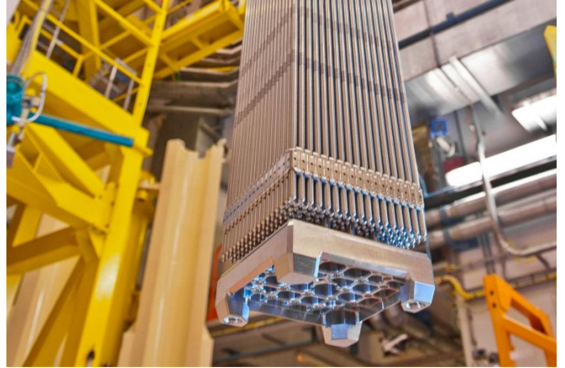
GAIA PROtect Enhanced Accident Tolerant Fuel (EATF) PWR fuel assembly (Framatome)
