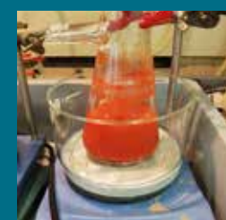
Mercury precipitation to cinnabar
