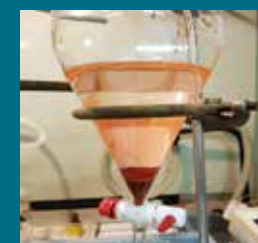
Cinnabar filtration in the treatment solution
