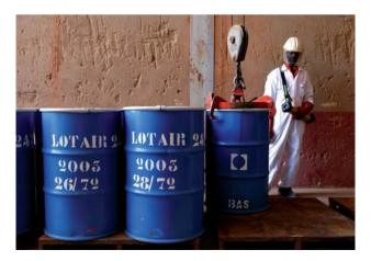
Filling circuit for yellowcake drums at the Somaïr ore processing plant, Niger
