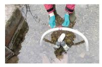
In 2012, Environmental R&D launched a research program, in partnership with the Université de Bruxelles in order to use the tool primarily for the measurement of the total uranium dissolved in solution, as well as to measure other contaminants of interest. DGTs were tested and optimized in the laboratory under controlled conditions. In a second phase, they were also successfully deployed on several mining sites, for use both in surface waters, as well as in porewaters from sediments.
