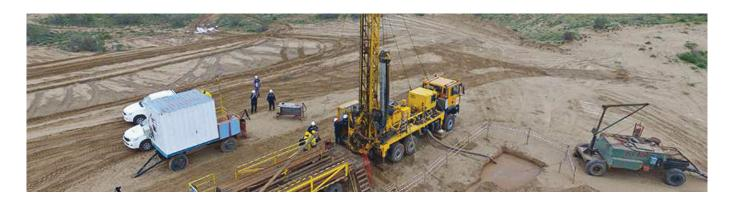
Development of the two mining sites, located approximately 60 kilometers apart, started in April 2004 after the signature of agreements between the two shareholders The in situ recovery (ISR) technology was chosen to solubilize the uranium directly in the rock.
