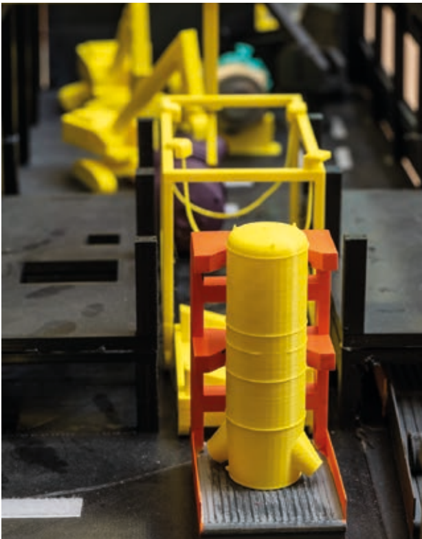
▲ Mockup of the dismantling project for the Georges Besse plant, Tricastin
