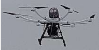
Hylium Drone (LH2 + Fuel Cell)
