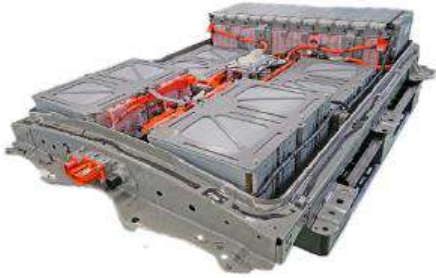
Battery pack, with its wiring, composed of modules
