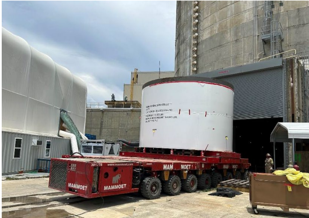
Image: The custom-built transport package on the transfer trailer for movement to the onsite temporary storage facility.
