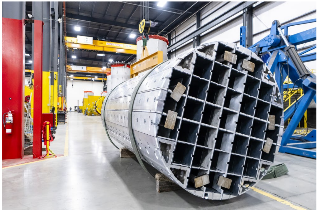
The EOS internal basket is efficiently assembled without welding before being placed inside the canister.
