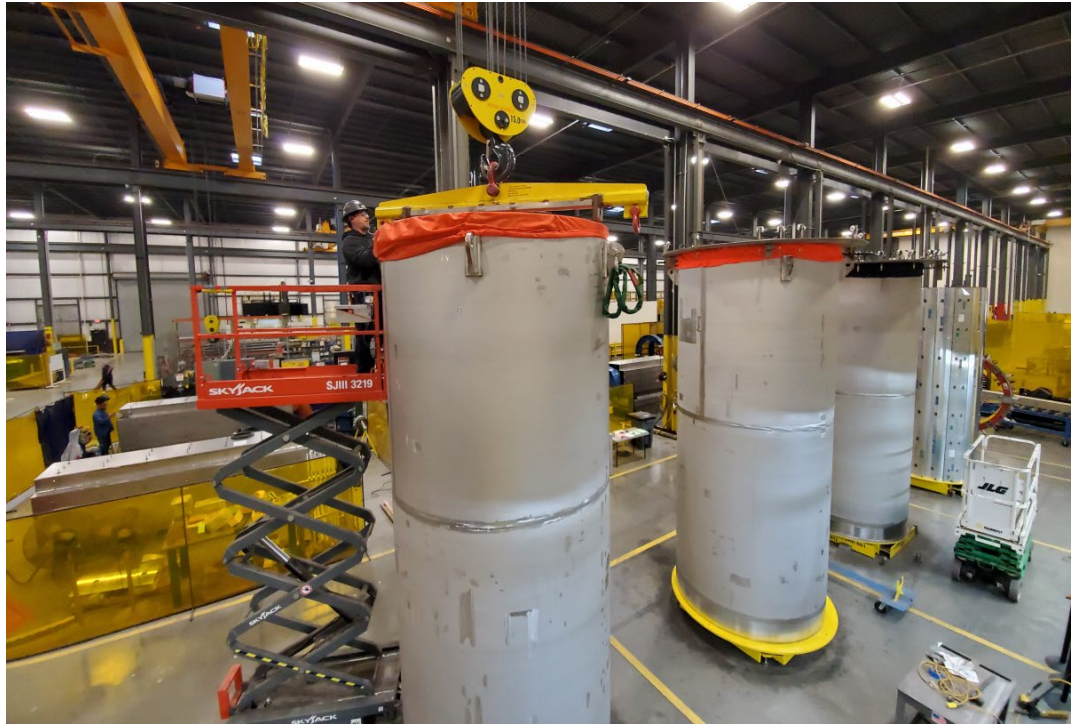
An employee adjusts the overhead crane's lifting yoke for moving a NUHOMS EOS canister within the TNF Kernersville facility.
