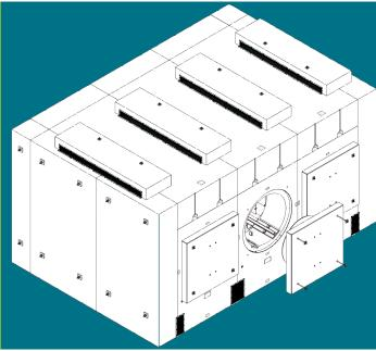
Ambient air enters the EOS HSM through ventilation inlet openings on both sides of its lower front wall. Air exits through outlet openings on each side of the top. The passive cooling system preserves fuel cladding integrity by maintaining spent fuel assembly peak cladding temperatures below acceptable limits during long-term storage.
