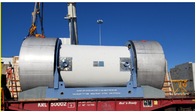
MP197HB cask preparing for rail shipment
