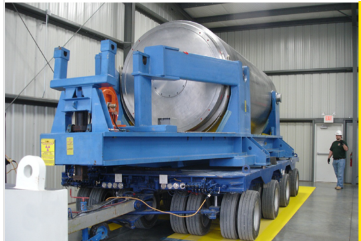
DSC Transfer Cask on Transfer Trailer
