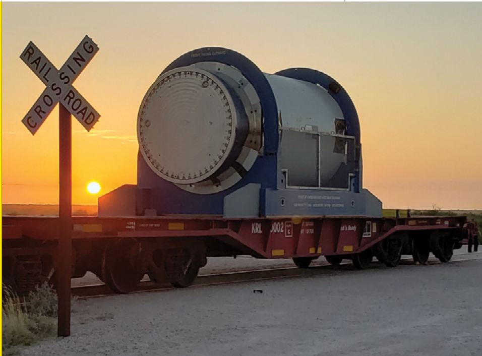
The MP197HB cask traveling by rail
