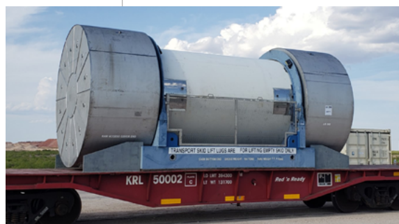
The MP197HB Cask on rail car ready for shipment
