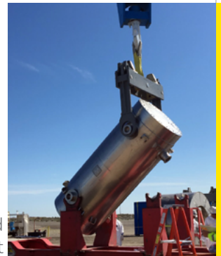
The TN RAM cask being placed horizontally for transport
