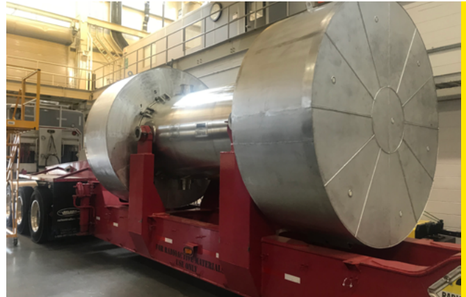
The TN RAM cask after loading
