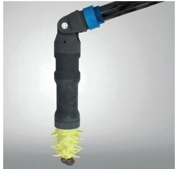
Anemone sampling tool installed on a pole
