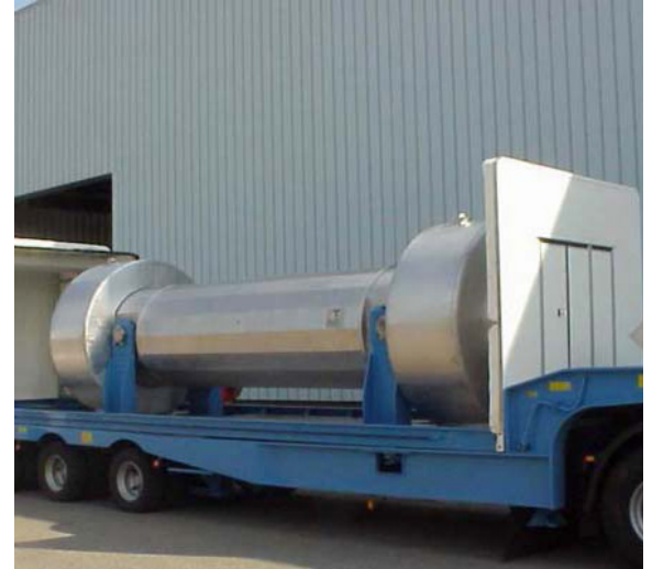
The TN 9/4 cask was licensed for damaged fuel transportation in France and Switzerland.
