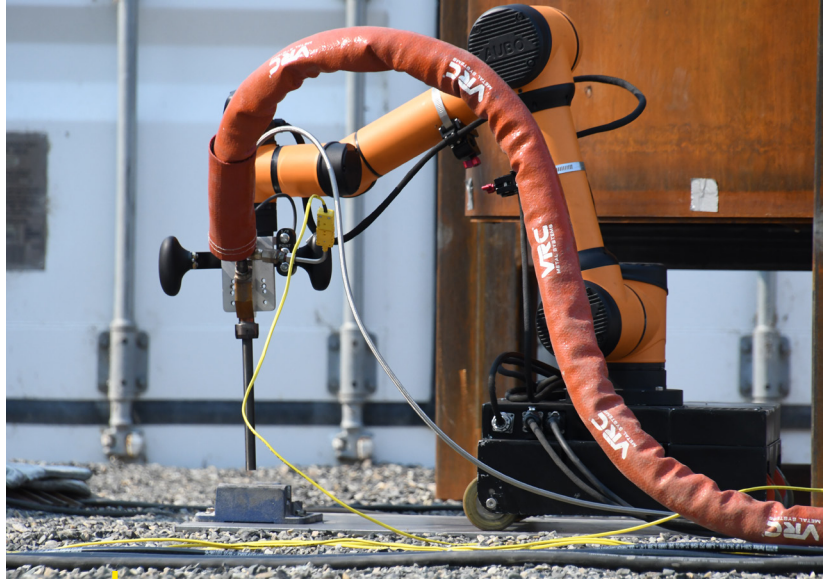
Cold spray robot with pre-demo test coupon
