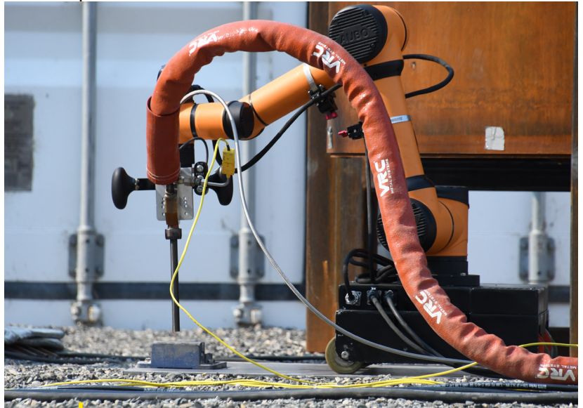
Cold spray robot with pre-demo test coupon
