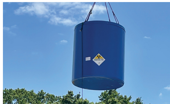
Standard resin liners collect the activity for disposal as low-level waste
