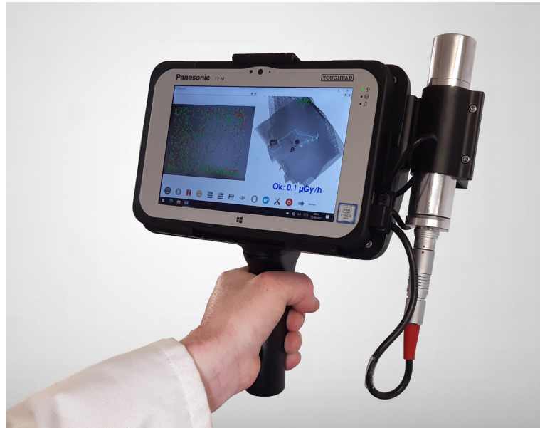
The MANUELA handheld metrology and radiological mapping tool
