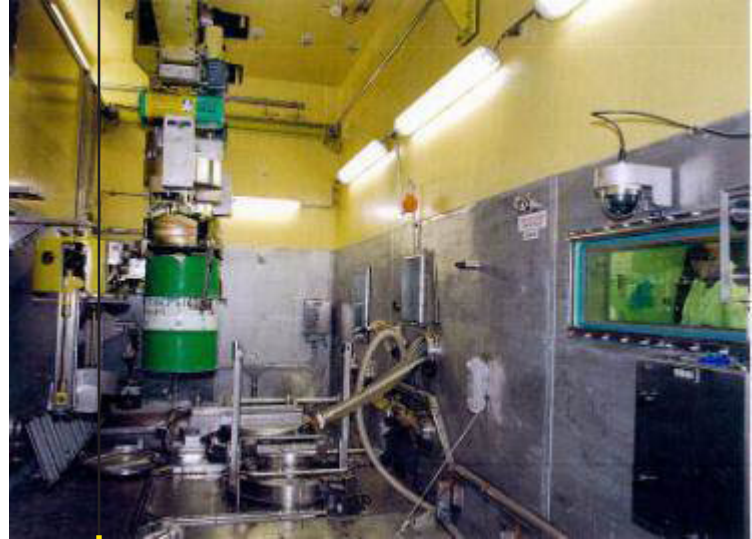
Repackaging in mobile hot cell
