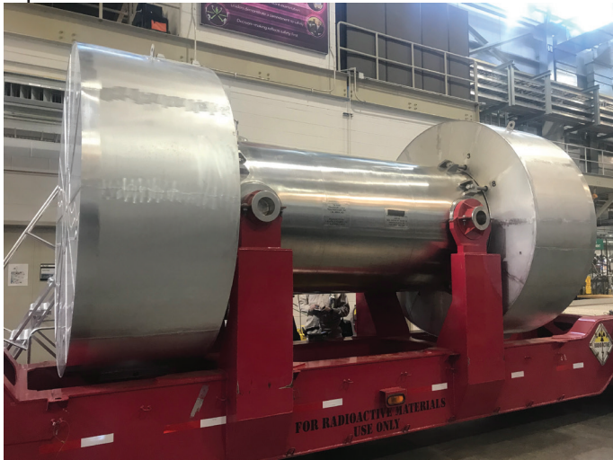
Loaded TN-RAM cask being prepared for transport to disposal site
